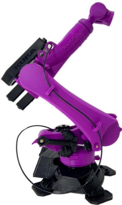
A 3D Printed Articulated Kuka Robot arm.
