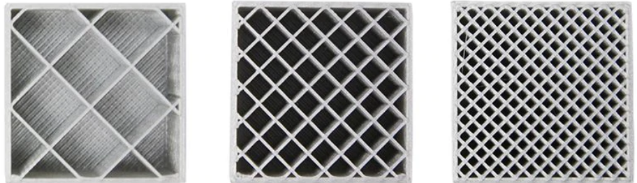
Image comparing 'grid' infill pattern at 5%, 10% and 20%
